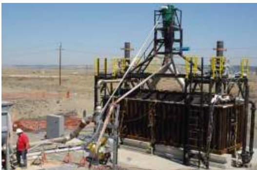
In-Container Vitrification Process
